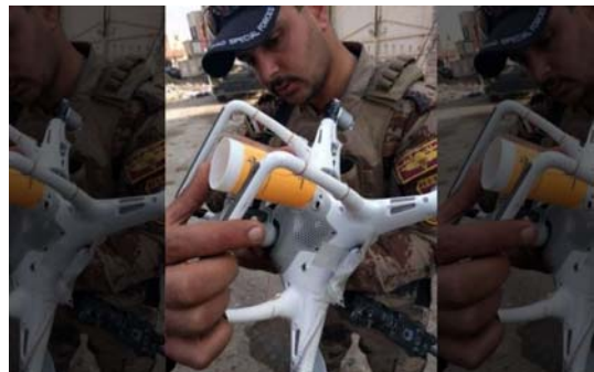
Iraqi Counter Terrorism Service soldier in Mosul examines an ISIS drone modified to carry a 40mm rifle grenade in the attached plastic tube. Grenade is dropped when the drone is over Iraqi forces. (Mitch Utterback)
